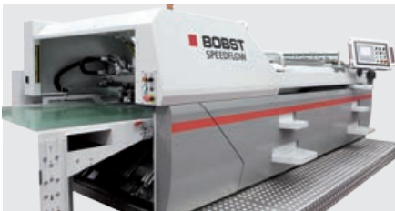
LEMANIC® SPEEDFLOW This module is part of the delivery section and enables optimal collecting of finished products at maximum production speed on all LEMANIC® lines.
