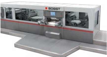
LEMANIC® FCC In a market where blanks are frequently changing shapes and dimensions, the flat-bed cutting process provides the necessary flexibility along with cost-effective tooling and operation.
