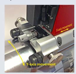
The X/Y MICRO ADJUSTERS have been devel- Exact Y-positioning: The Y-axis adjustoped to allow users to move the analysis head ment turns the wheels of the AniCAMs of the camera laterally up to 10 mm (±5 mm) feet. As a unique feature this assures a along the x-axis and across the y-axis by turn- constant distance of the whole measuing the feet to assist in finding special engrav-ring area to the camera - regardless the ings.
