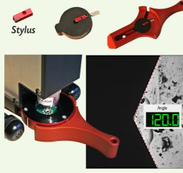
Stylus angle measurement: Simple stylus mount and software to check the angle and condition of the stylus. The hardware mount supports OHIO, HELL and MDC styluses. The software allows the visual representation of the stylus for condition and to measure the angle to ±0.1 degree.
