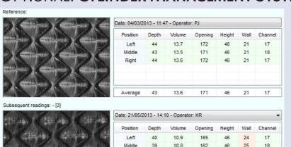
The CMS application can ideally be used to analyse the wear of all cylinder.s in the inventory.
