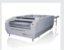
Digital washer with flat and round brushes in large format. Equipped with double tank which allows to separate the black layer of the digital plates from the washout solvent. Automated brush height setting for optimum brush pressure according to the plate thickness. Temperature control of the washout solvent and integrated solid content measurement.
