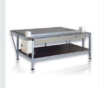
Fast, precise and safe cutting of foil based plates with clean burr free edges. A clamp opening up to 8 mm (0.31") allowing space to easily manoeuvre all plate thicknesses. A cutting blade and clamp that is operated by compressed air. Cutting angle 90°. Two handed operation for optimum safety.
