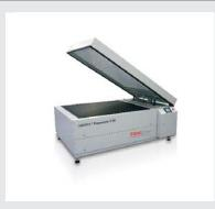
Large size exposure unit with a cooled metal bed for back and main exposure. Operating status of each tube is monitored, operating hours are recorded and defective tubes are displayed. The unit includes a temperature control unit, a touch screen for user friendly operation and 20 memory settings. Exposure lid opens automatically. New generation of electronic ballasts, which double lamp life compared to conventional ballasts.
