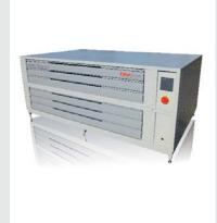
High heat output for reaching quickly the optimal temperature in six easily accessible drying drawers. Two separate drying sections provide uniform temperature distribution, the efficient exhaust system prevents solvent vapours to escape – even when opening the drawers. Including digital timers with audio signal to indicate the end of the drying process.
